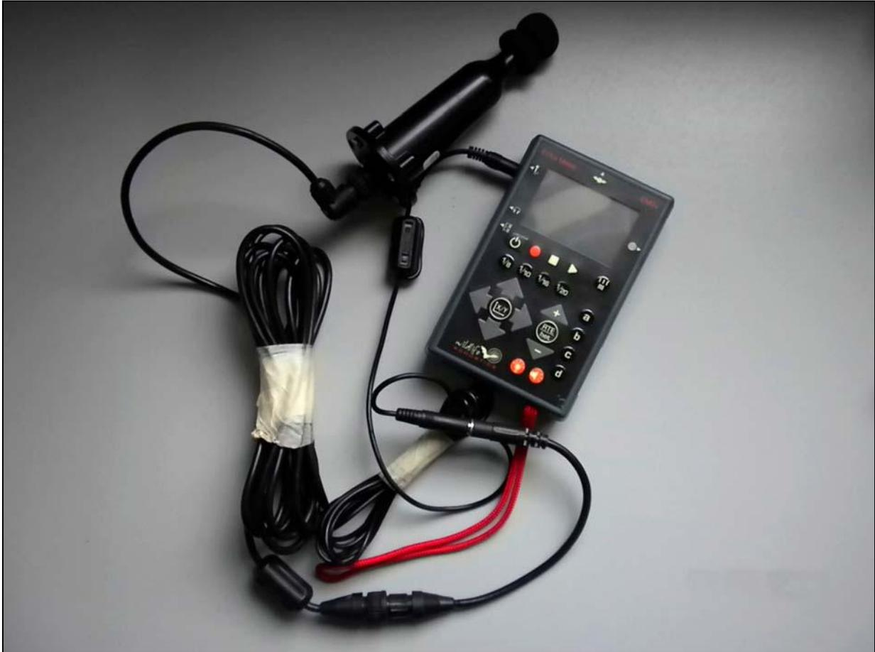
Figura 2.2 - *Bat detector* modello EM3+ (*Wildlife Acoustics, Inc.*, 2011) con microfono SMX-UT (*High Performance Ultrasonic Microphone*).
