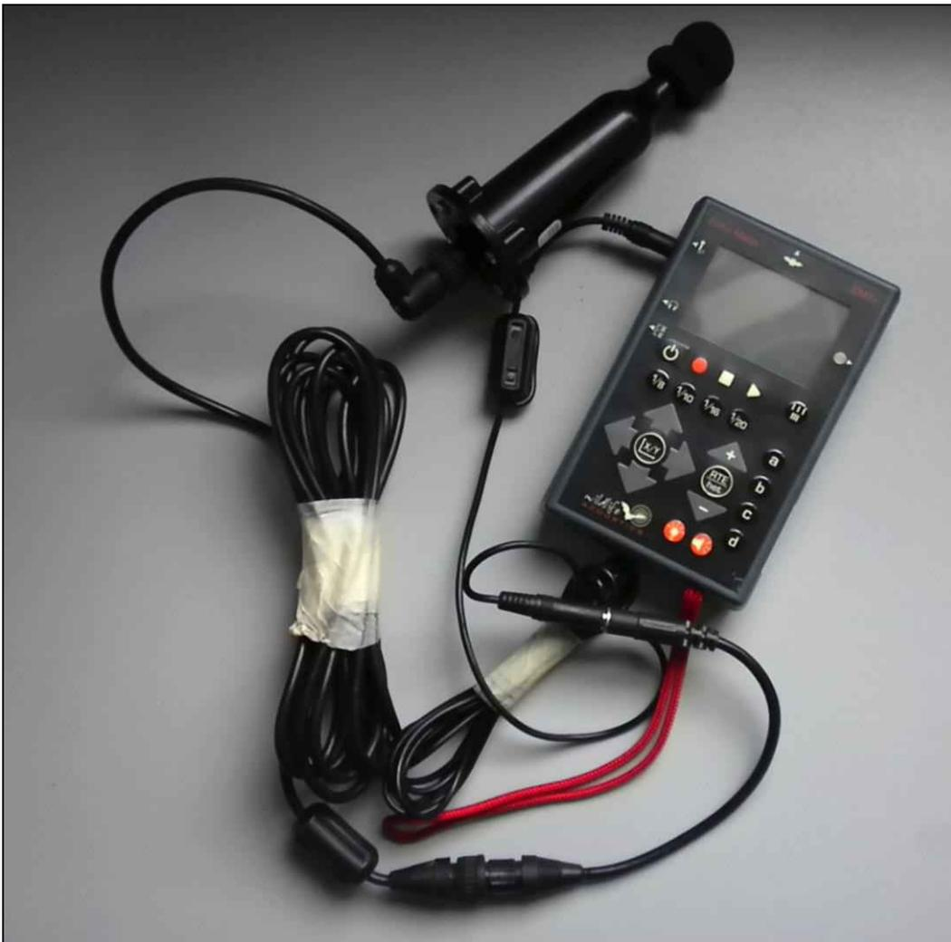
**Figura 2.1 - Bat detector modello EM3+ (Wildlife Acoustics, Inc., 2011) con microfono SMX-UT (High Performance Ultrasonic Microphone).**
